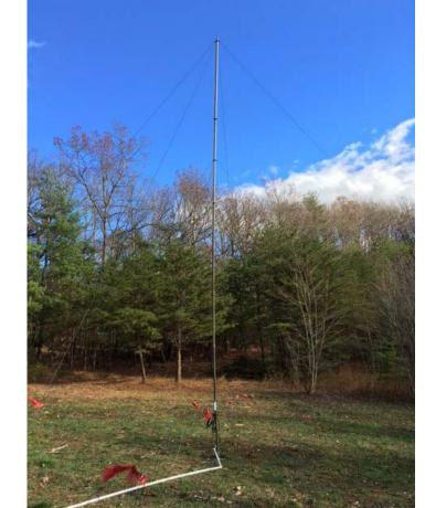
Only needs 8 ground stakes, and flags and chimes to keep out critters. Lowest part of loop is ~4' above ground. Has withstood 50 mph winds already.
